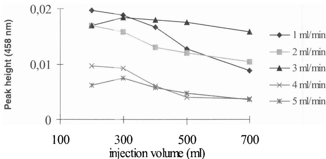
Figure 2. Effect of sample injection volume on peak height absorbance measurements at 458 nm, for a coprostanol concentration of  $4.5 \times 10^{-4}$  M, established at different carrier flow-rates: (◆) 1, (■) 2, (▲) 3, (×) 4, and (※) 5 mL.min<sup>-1</sup>.
