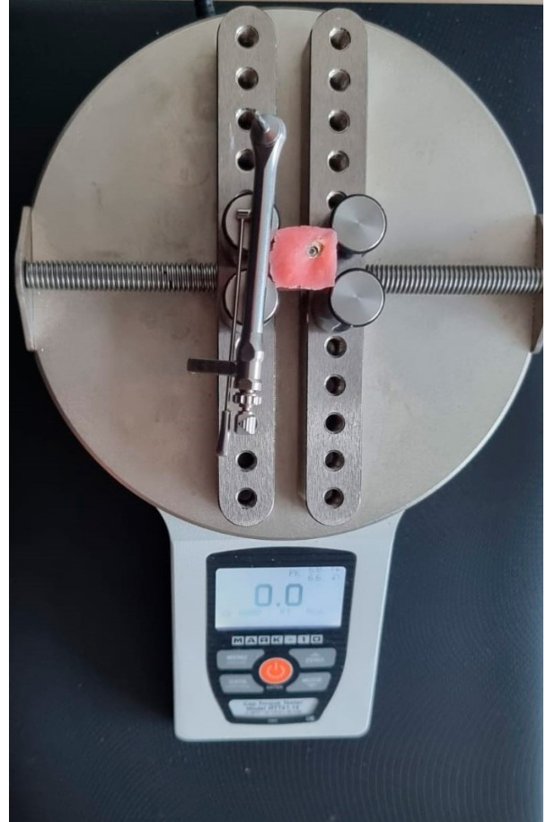
FIGURE 3. Biomechanical reverse torque device (Mark 10, NY, USA)
