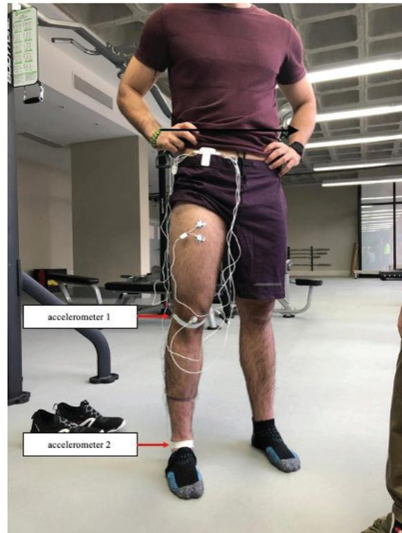
Fig. 1. Location of accelerometers.
