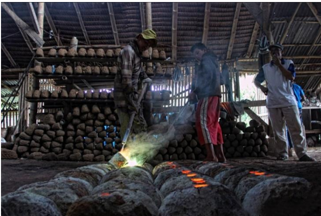
Figure 1: Pouring Brass Liquid into the Mold
