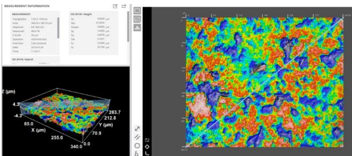
Figure 3: Result of investigation of hybrid polished ceramic samples after application of Double flow (PetroDent, Russia) powder.
