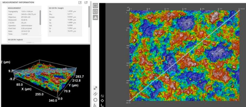
Figure 4: The result of the study of hybrid polished ceramic samples after the application of Flow-Clinz-Pro powder.
