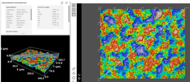
Figure 5: Result of investigation of hybrid polished ceramic samples after application of Omniflow (OMNIDENT, Germany) powder.
